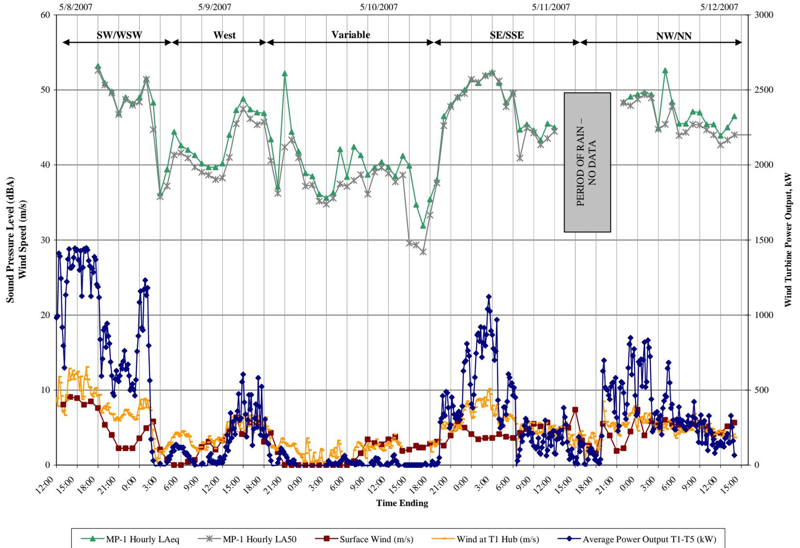
Figure 7-2. Sound Levels at MP2 in Relation to Wind Turbine Power Output and Wind Speed
