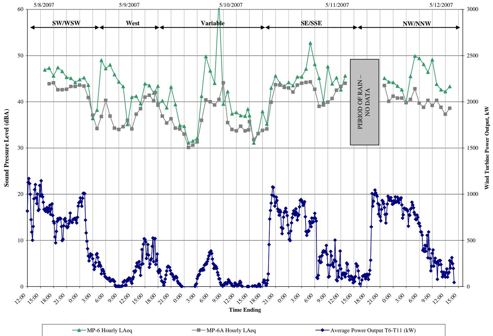
Figure 7-11. Sound Levels at MP5 and MP-7 in Relation to Wind Turbine Power Output and Wind Speed
