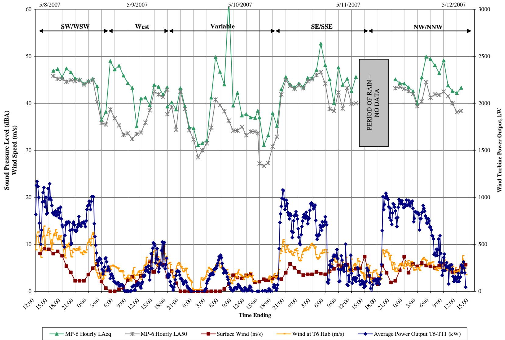
Figure 7-6A. Sound Levels at MP-6A in Relation to Wind Turbine Power Output and Wind Speed
