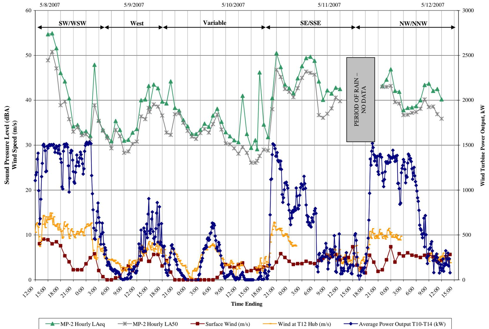
Figure 7-3. Sound Levels at MP-3 in Relation to Wind Turbine Power Output and Wind Speed
