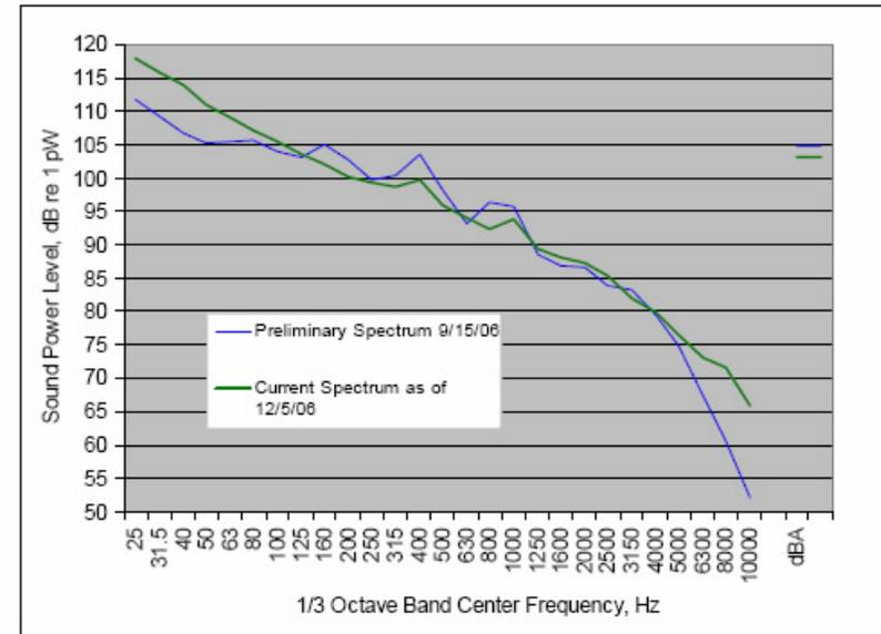
**Figure 2.2.1** Preliminary and Current 1/3 Octave Band Sound Power Level Spectrum for the Clipper C96 Wind Turbine (from Prototype Field Measurements)
